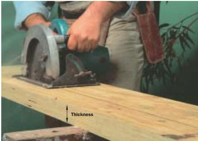
Rip sawing through the thickness.
